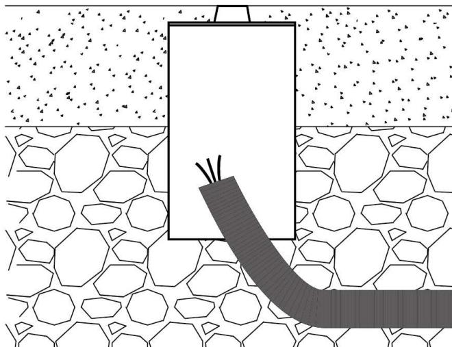
UL/CUL : for pool or SPA use, luminaire shall be installed in a non-metallic forming shell only
